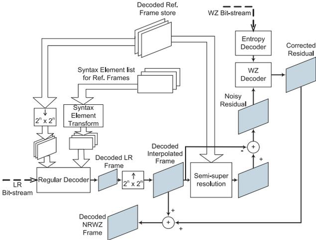
Figure 3. Architecture for the NRW decoder
