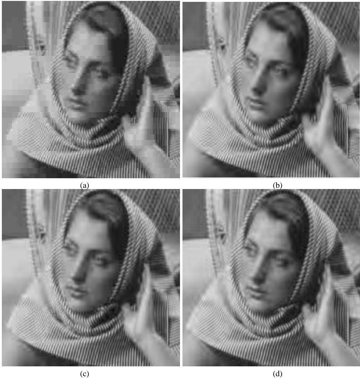
Fig. 8. Detail of image Barbara compressed at 0.3 bits/pel. (a) DCT, (b) wavelets, (c) 8x16 GLBT, (d) 8x48 GenLOT.
