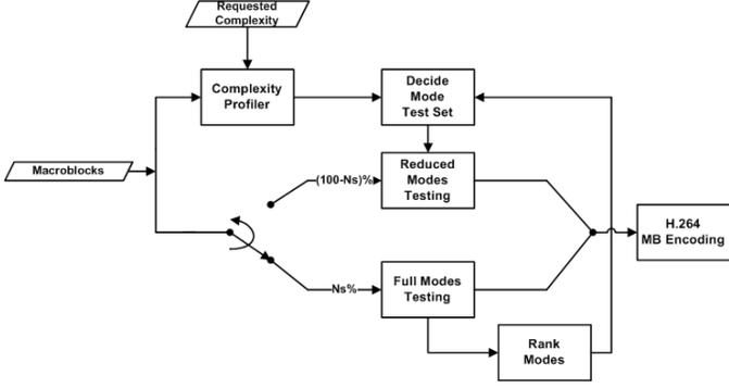
Fig. 2. Complexity control framework.
