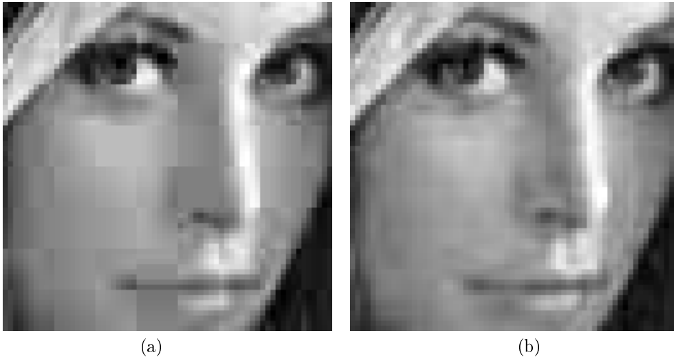
Figure 5: Zoom of image compressed using JPEG at 0.5 bits/per pixel. (a) DCT, (b) LOT.
