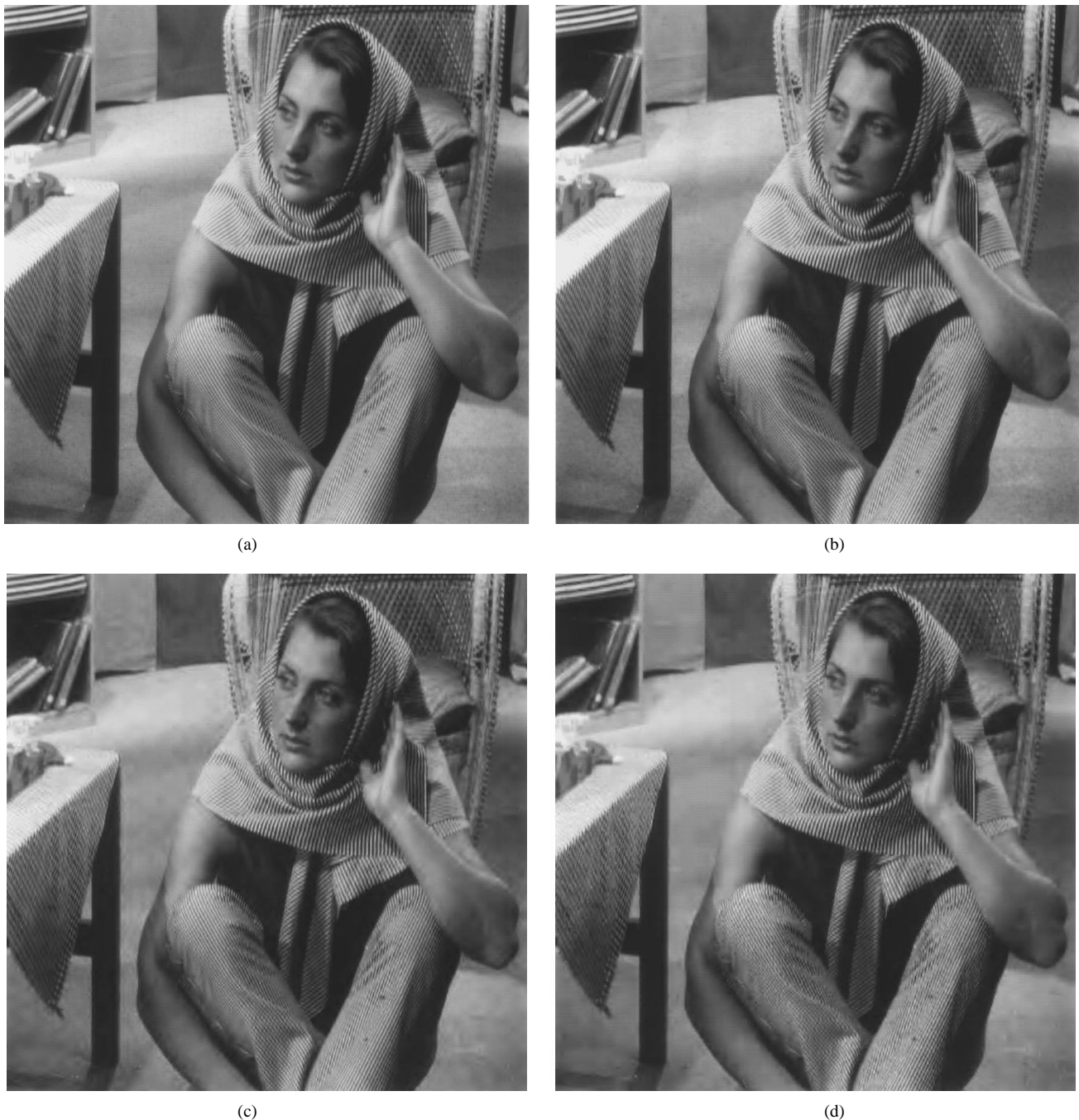
Fig. 4. Subjective evaluation of DWT-JPEG, using S = 3 . Filter bank and bit rate are indicated. (a) Original, (b) 1.0 b/p—B11/13, (c) 0.5 b/p—B11/13, and (d) 0.5 b/p—B3/5.
