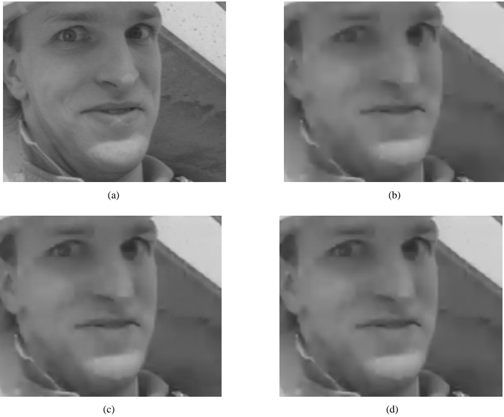
Fig. 10. (a) Original frame. (b) Non-key frame without enhancement. (c) Enhanced sequence with regular block motion compensation. (d) Enhanced sequence with overlapped block motion compensation. This Figure can be better visualized in the electronic version.
