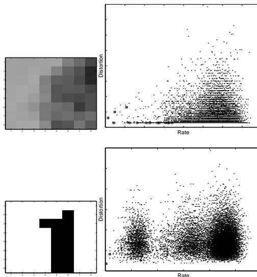
Figure 4. Sample blocks for the simplified experiment and the corresponding 64K RD plots. RD points obtained by block thresholding are marked.
