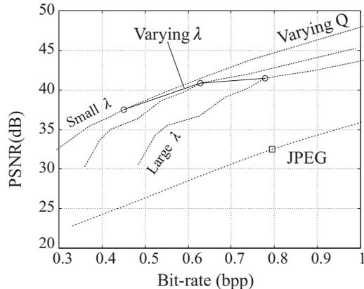
**Figure 6. PSNR plots for MRC and JPEG.**
