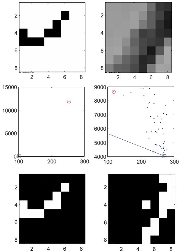
**Figure 5. Sample blocks, RD plots for block thresholding and resulting Mask blocks. The operating slope is indicated along with the best RD point (□) and the RD point for a uniform mask (○).**
