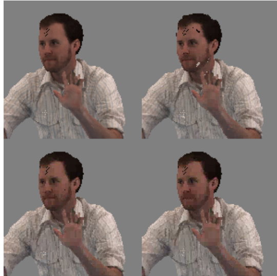
Fig. 5. Front projection rendering comparison of frame 58 in sequence “man” at 3.7 bpv. Original, MCIC, MCIC designed under a projection-based distortion metric, RAHT.
