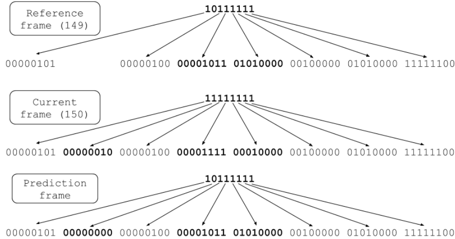
Fig. 2. First two levels of the octree representation of frames 149 and 150 in point-cloud sequence Man [9], and octree prediction for frame 150 using frame 149 as reference. Corresponding levels in the frames’ octrees which are different are indicated in bold typeface.
