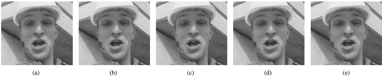
Fig. 6. Details of the Foreman sequence:(a) high resolution frame encoded with H.264, (b) Lanczos interpolation from an H.264 encoded low resolution frame, (c) PDSSR of the previous case, (d) DCT interpolation from an H.264 encoded low resolution frame and (e) TDSSR of the previous case.
