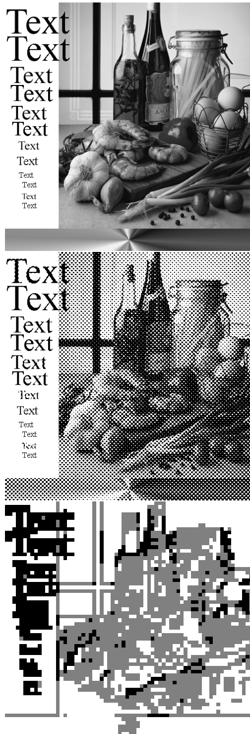
Figure 2. (a) Enlarged Sample Mixed Image wine , (b) its halftone and (c) correspondent classification map (with T_{i_o} = 30 and T_{h_i} = 120 ). (white=smooth, gray=detailed, black=edge).
