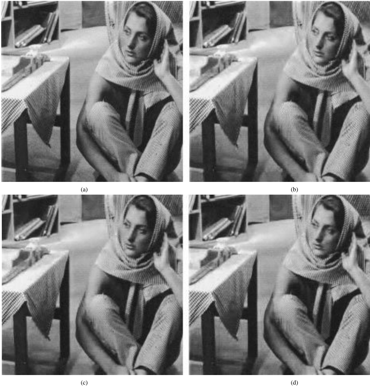
Fig. 15. Embedded coding results of Barbara at 1:32 compression ratio. (a) Original image. (b) SPIHT, 27.58 dB. (c) Embedded 8 \times 16 GLBT, 29.04 dB. (d) Embedded 16 \times 32 GLBT, 30.18 dB.
