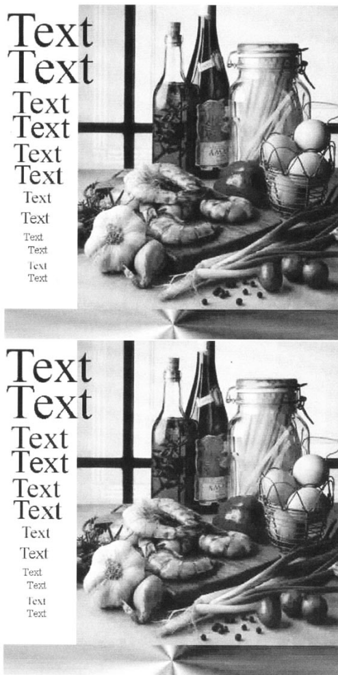
Fig. 8. Image "mixed" after compression to 0.52 b/pixel. Top: regular. Bottom: using proposed HVQ-analyzer-based system.
