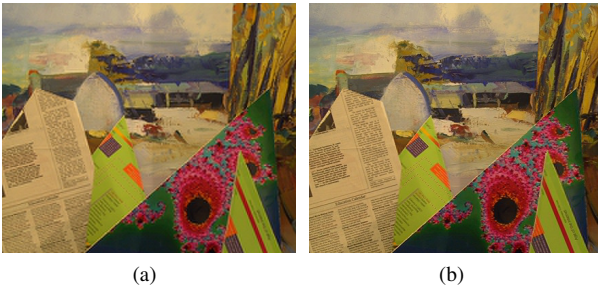
Figure 5: Barn1 sequence, view 1: (a) DCT-based up-sampled image (27.49 dB) and (b) DCT-based SR image (36.22 dB).
