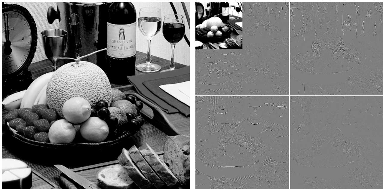
Figure 1: Pictorial depiction of a two-level wavelet transform
