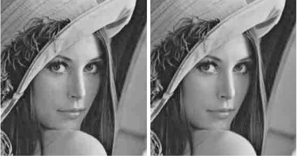
Figure 5 –Zoom of reconstructed image after compression using the regular quantizer design method at 25:1(left). Same result for using the proposed design method is shown on the right.
